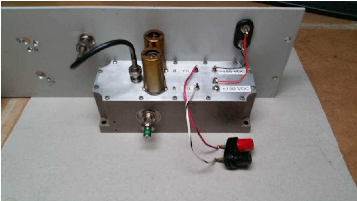
Figure 1 – 5722 diode noise generator, two tubes in parallel.
